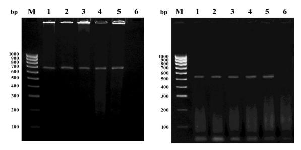
Figure 2: Amplification products (670 and 517 bp) generated with the *M. javanica* species-specific Fjav/Rjav (A) and MJ-F/MJ-R (B) SCAR primers, respectively. M: 100 bp DNA Ladder, 1-5 *M. javanica* isolates 1: El-Badary, 2: Manfalout, 3: Sedfa, 4: Sahel-Selim, 5: El-Fath and 6: water as a negative control (PCR reaction without DNA).
